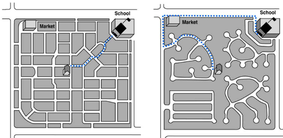
**Figure 1: Shorter trip distance with connected network**
